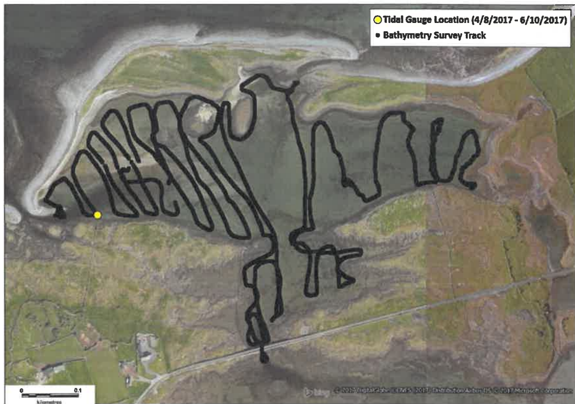
Figure 2.1: Bathymetric survey lines of the vessel and location of tidal gauge.
